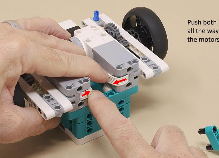
Push both motor wires all the way up against the motors.
