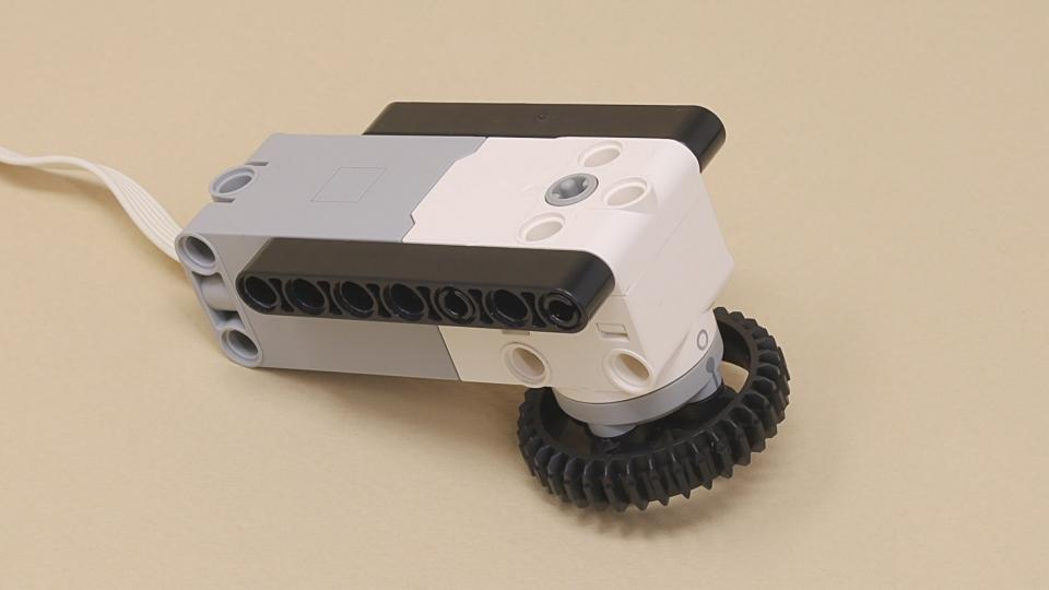
Place the motor so the gears mesh, aligned straight, keeping the motor in its zero position.
