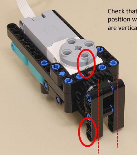
Check that the motor is in its zero position while the turntable beams are vertical as shown.
