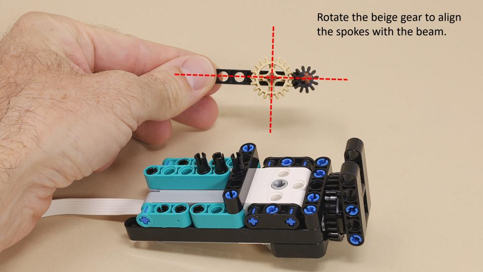
Hold the turntable beams to keep them vertical as shown while inserting the gear axles.
