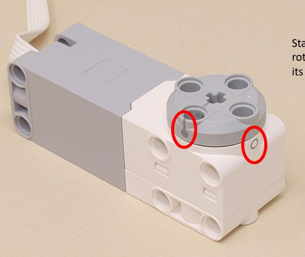
Start with this motor rotated 90 degrees from its zero position as shown.
